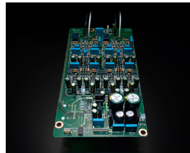
Balanced, dual mono optical phono stage
