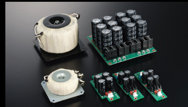
Power transformer for main drive stage (top left) Power rectification circuit for main drive stage (top right) Power transformer for pre-drive stage (bottom left) Power rectification circuit for input stage (bottom center) Left and right power rectification circuits for pre-drive stage (bottom right)
