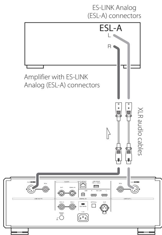
Use XLR audio cables to connect the analog audio output (XLR/ESL-A) connectors on this unit to an amplifier that has ES-LINK Analog (ESL-A) connectors.
