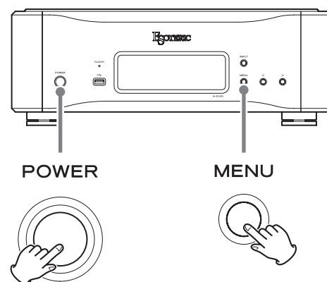
Settings are retained even if the power plug is disconnected. Follow these procedures to restore the factory default settings and erase all changes in memory.
